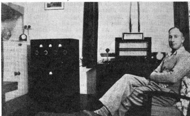
If you hear or work ZL1GW, Arapui, New Zealand, this is a view of the station and its operator. He is a 28 mc man with a 3-element beam and a 3-stage 100-watt transmitter using an HK54 final; the Rx is a 361A.
