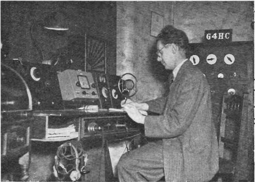
G4HC, Colchester, runs a 25-watt outfit, CO 6V6-807, with an HRO receiver and 6J7-6C5-P/P 6L6 modulator; the aerial is as described in our issue for February, 1939. G4HC is unusual in that AC is obtained from a 400-watt rotary converter run off the DC supply.
